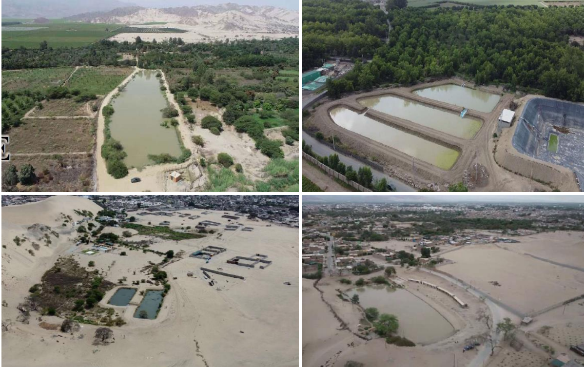
Figure 16. Artificial recharge ponds (pozas) in the Ica Valley, built to facilitate managed artificial recharge (MAR).
